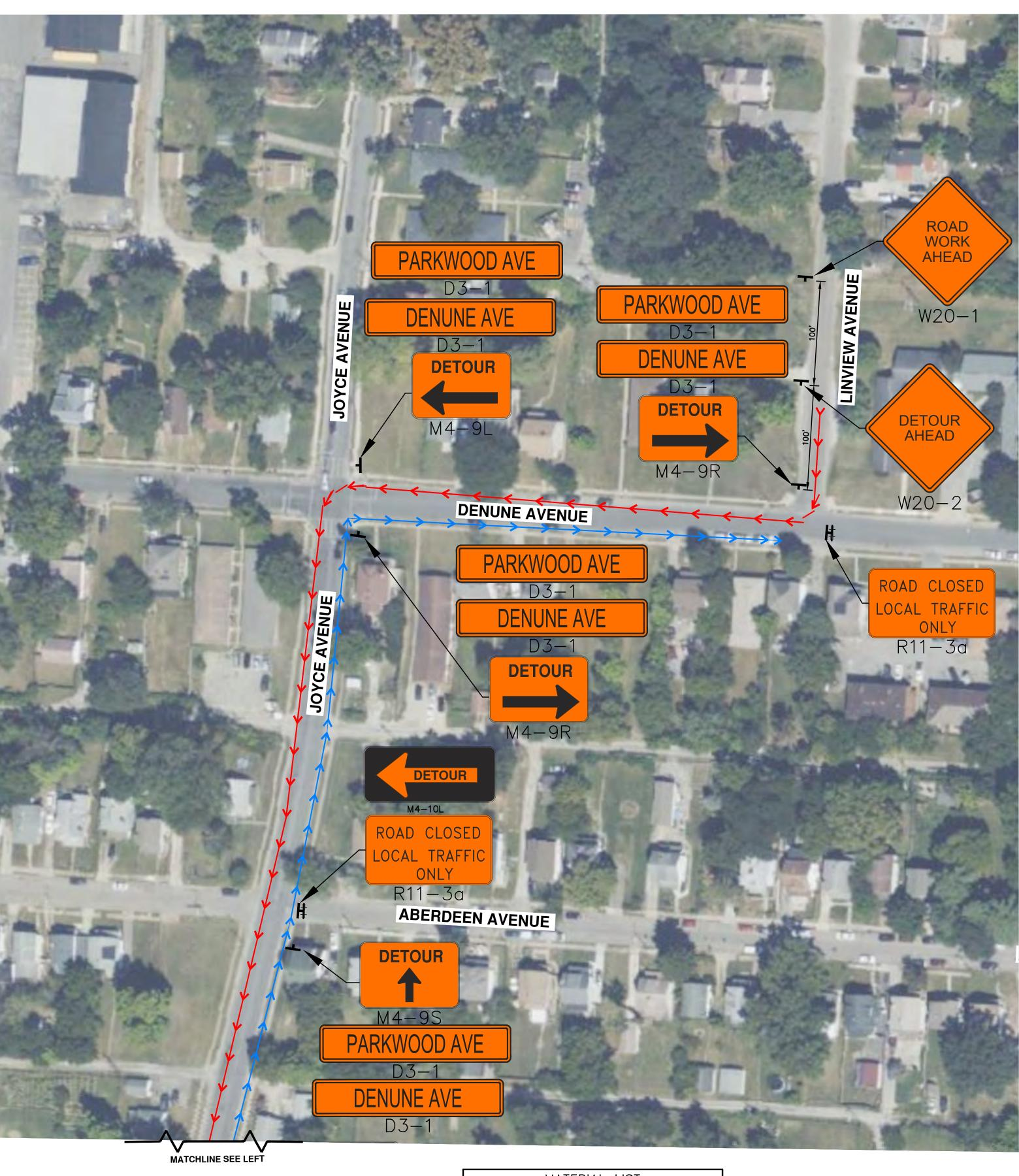
MATERIAL LIST CODE: QTY: STREET NAME D3-1 14 DETOUR - LEFT ARROW M4-9L 2 DETOUR - RIGHT ARROW M4-9R DETOUR - STRAIGHT M4-9S ARROW DETOUR - LEFT ARROW M4-10L ROAD CLOSED LOCAL TRAFFIC ONLY R11-3A ROAD WORK AHEAD W20-1DETOUR AHEAD W20-2
